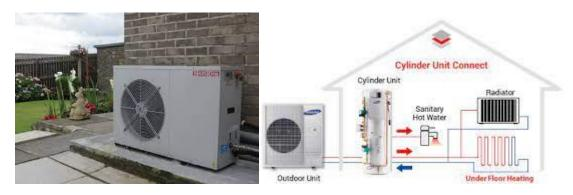
A Heat Pump works like a refrigerator in reverse – instead of cooling the inside of your fridge and emitting that heat via the back of the fridge into the room, it effectively takes heat from outside (even in cold weather) and uses that to heat hot water tank(s) to give hot water for radiators, showers etc inside the home.
